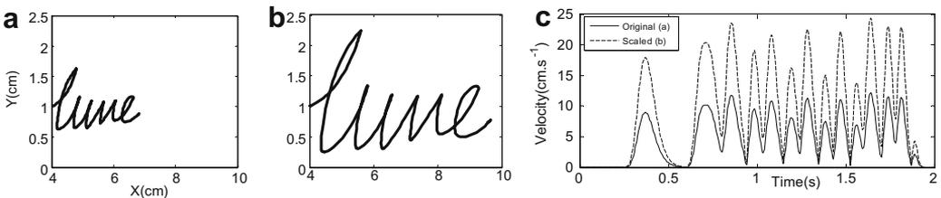
**Fig. 2.** Global effects, both in the trajectory and the velocity spaces, of a 100% increase ( $k_i = 2$ ) in the parameters  $D_i$ . Note that the time scale of the velocity profiles remains stable in this case, i.e., the time scale is preserved.
