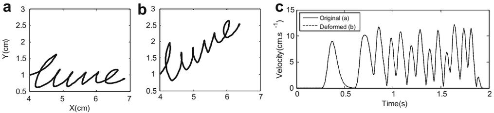
Fig. 3. Global effects, both in the trajectory and the velocity spaces, of a 35° increase in the direction parameters ( $\theta_{di}, \theta_{fi}$ ). Note that there are no predicted effects on the velocity profiles, i.e., both the time and space scales are preserved.
