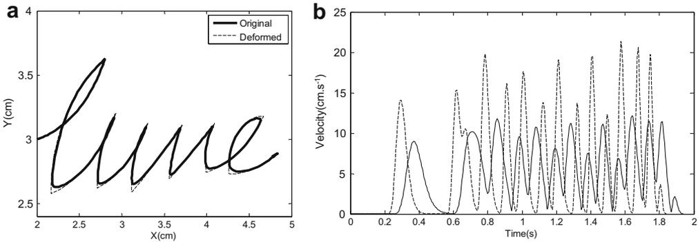
**Fig. 5.** Global effects, both in the trajectory and the velocity spaces, of a decrease in the parameters  $\mu_i$  by about 10% of their original values, which leads to a sharper pattern (the same effect is observed when decreasing the parameters  $\sigma_i$ ).
