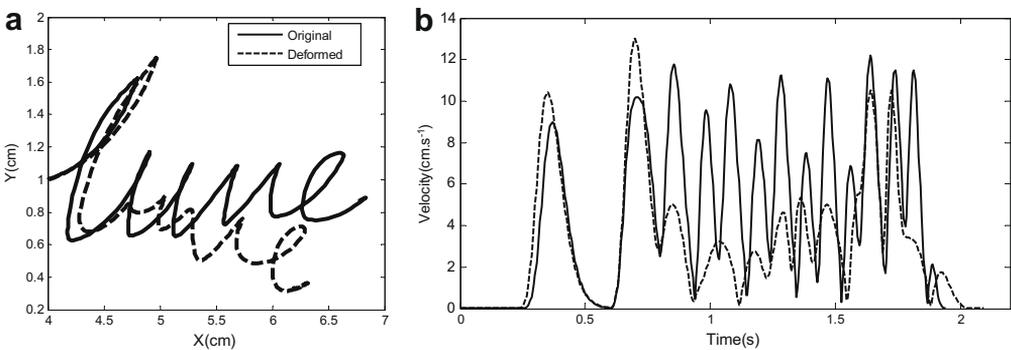
**Fig. 6.** Local variational effects of the Sigma-Lognormal parameters, both on (a) the trajectory and (b) the velocity profiles, when all the parameters are varied slightly.
