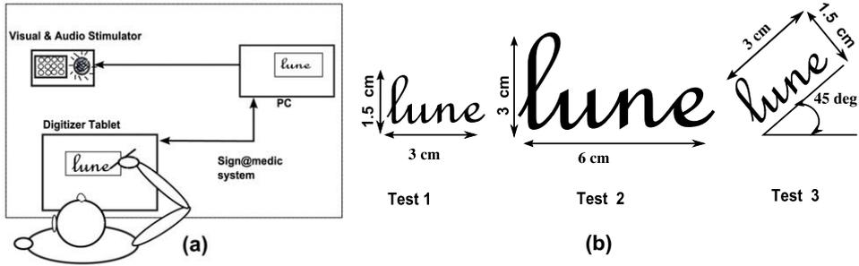
**Fig. 7.** (a) illustration of the apparatus and the experimental protocol used in the acquisition of handwriting. After receiving an audio stimulus, the writer writes a word in the specified rectangle, and the digitizer records the corresponding trajectory of the stylus; (b) illustration of the three tests used in this experiment.
