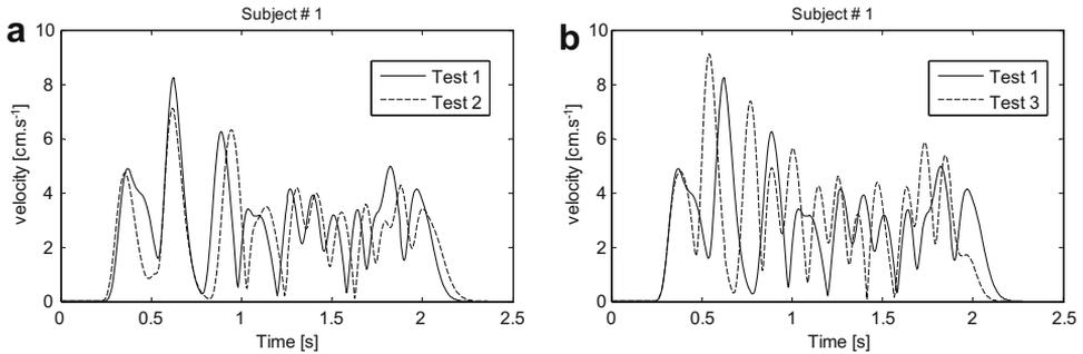
**Fig. 12.** Typical superposition of velocity profiles corresponding to the fiducial patterns constructed from the (a) *Test*<sub>1</sub> and *Test*<sub>2</sub>, and (b) *Test*<sub>1</sub> and *Test*<sub>3</sub> data of a writer #1, after normalizing the scale (using Eq. (5a)). The time scale is more or less locally preserved, depending on the residual local variability of the parameters.
