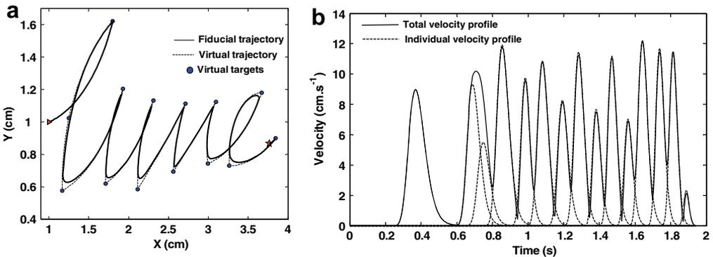
Fig. 1. A typical modeling with Sigma-Lognormal parameters of: (a) the handwriting pattern of “lune”; and (b) its corresponding velocity profile. Note that the word has been built with 14 strokes, 13 of which represent the main pattern and the last stroke depicting the antagonist neuromuscular effect that appears at each end of a movement.
