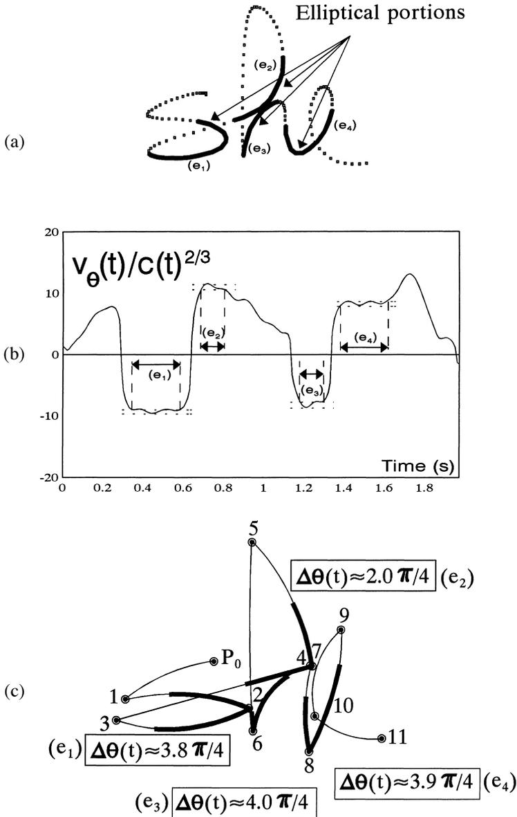
Fig. 4. Real handwriting produced by a human subject and analyzed with the Vectorial Delta-lognormal Model: (a) original word with highlights on the elliptical portions; (b) the ratio  $v_{\theta}(t) / c^{2/3}(t)$  as a function of time; (c) segmented overlapping strokes as extracted from analysis-by-synthesis and regions of superimposition where conditions apply.
