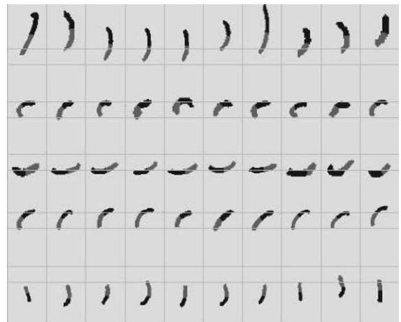
Fig. 4. Each row shows some examples of segments belonging to the same cluster. For each row, the two horizontal lines indicate the core zone, which is automatically extracted from the word image. The temporal orientation of the stroke is given by the two colors of each segment: light gray first.
