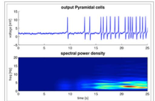
Simulation of a neural mass model showing network spiking during the onset of a seizure.<sup>[28]</sup> As the gain  $A$  is increased the network starts to oscillate at 3Hz.
